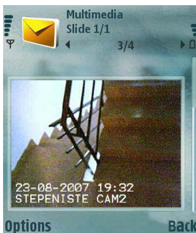
Fig. 4 MMS received by client's cellular phone displaying current image from targeted security camera.
